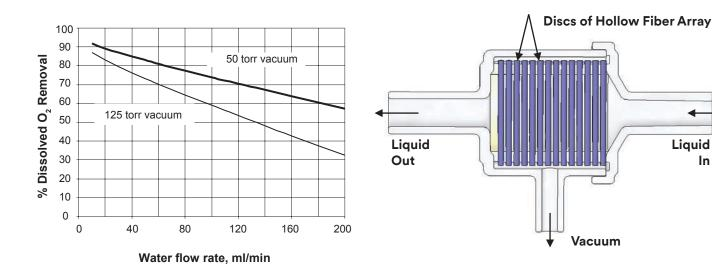
Curves represent nominal values generated using water on the shellside and vacuum on the lumenside at 20°C. Characteristics may change under different operating conditions.
