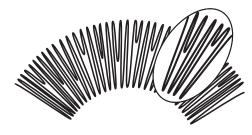
Conventional pleat designs, with fulldepth densely packed pleats, fill the upstream pleat surface with contaminant that quickly constrict flow at the pleat's inside diameter.
