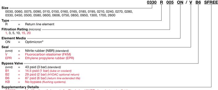
SO263 = Modification of elements for Skydrol or HYJET phosphate ester fluids SFREE = Element specially designed to minimize electrostatic charge generation
