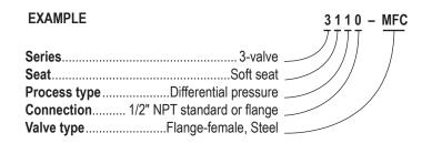
To meet all of your specific application requirements, the following **additional options** are available for these manifold valves. To order all or any of these options, simply add them to the part number as shown in the diagram below.
