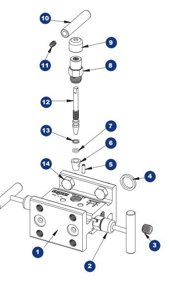
1 Valve body 2 Blue dust cap 3 Plug 4 Gasket ring 5 Slotted spring pin 6 PTFE back-up ring 7 Valve bonnet 8 Green dust cap 9 Valve "T" handle 10 Set screw 11 Valve stem
